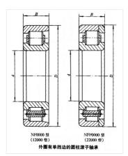
Bearing Model NF309/C3 Overall dimension (mm) d 45 D 100 D 100 B 25 Limit speed (RPM) Grease -Oil lubrication -Rated load Cr(N) -
