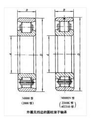
Overall dimension (mm) d 180 D 280 D 31 Limit speed (RPM) Grease -Oil lubrication -Rated load Cr(N) -
