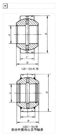
Bearing Model GE70XS/K Overall dimension (mm) d 70 d 70 D 110 B 58 Limit speed (RPM) Grease -Oil lubrication -Rated load Cr(N) -Cr(N) -
