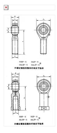
Bearing Model SIBP20S Overall dimension (mm) d 20 d 40 D 46 B 25 Limit speed (RPM) Grease -Oil lubrication -Rated load Cr(N) -
